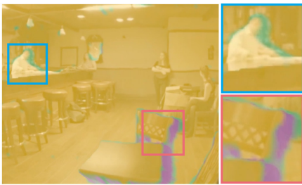
Fig. 16. Color-coded visualization depicting the use of our three-layer representation in a given frame for a displaced view (orange: foreground layer; green: extrapolated layer; purple: inpainted layer).
