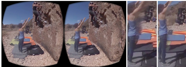
Fig. 6. Comparison of two different methods to modulate the opacity values \hat{\alpha}^F as a function of distance to the center of projection to obtain \alpha^F . Left: Original view as seen in the HMD. Right: Close-up of a displaced view with two different modulations: linear interpolation (left), and blending based on a logistic function (right). Aggravated ghosting results from using a linear interpolation as a function of distance.
