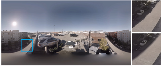
Fig. 5. Left: RGB panorama. Right: Corresponding inpainted layer obtained using a patch-based approach [43] (top), and our result using a spring metaphor-based method [5] (bottom). The patch-based approach produces local artifacts that are very prominent when visualized on an HMD. While the spring-metaphor inpainting yields a blurred approximation in the area to inpaint, for our application this smoothness is preferable.
